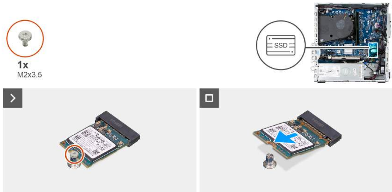
Figure 22. Removing the M.2 2230 solid state drive
