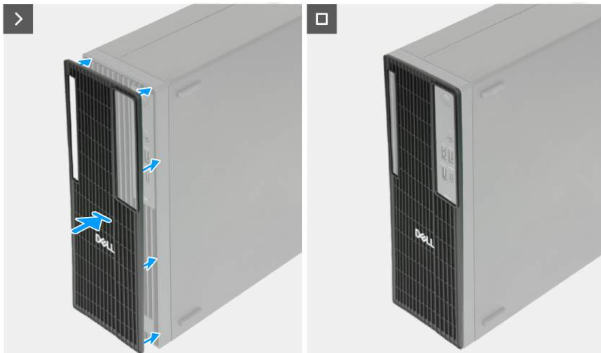
Figure 15. Installing the dust filter
