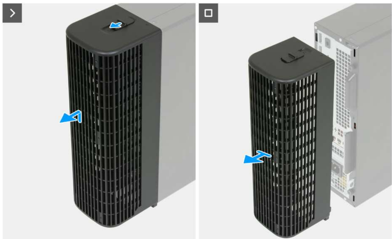
Figure 4. Removing the cable cover
