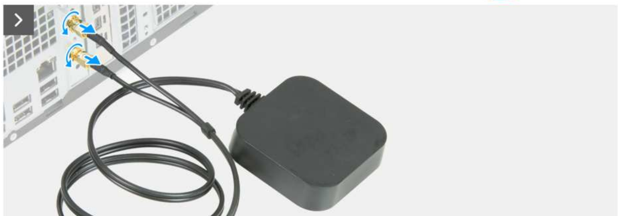
Figure 41. Removing the puck-antenna expansion card
