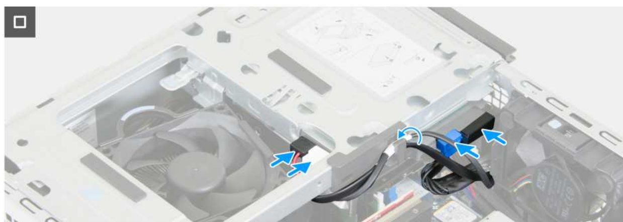
Figure 52. Installing the drive bay
