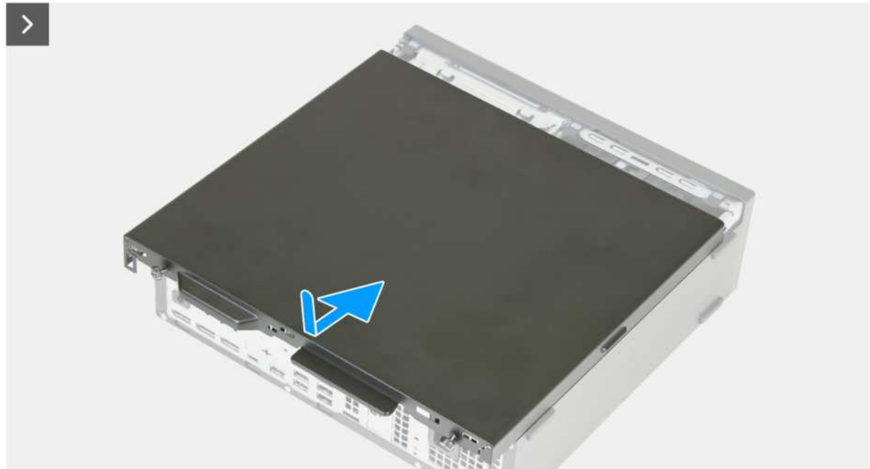
Figure 8. Installing the side cover
