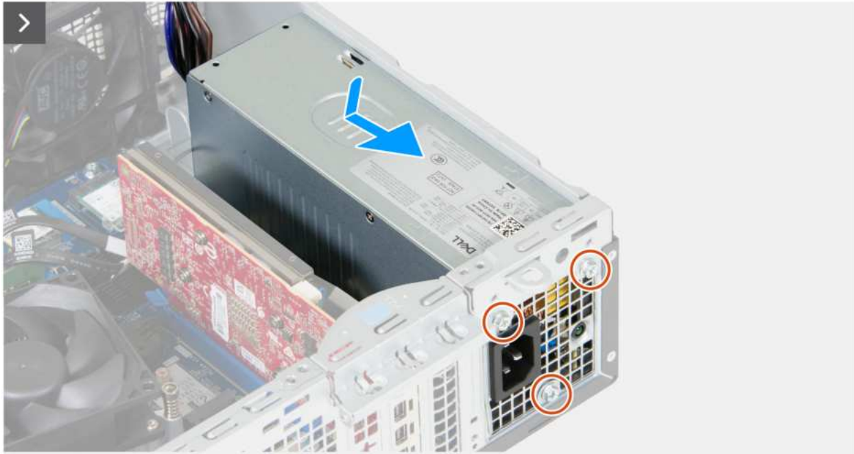
Figure 78. Installing the power-supply unit
