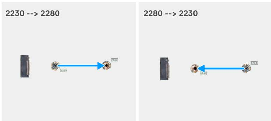
Figure 26. Moving the solid state screw mount on M.2 slot 0
