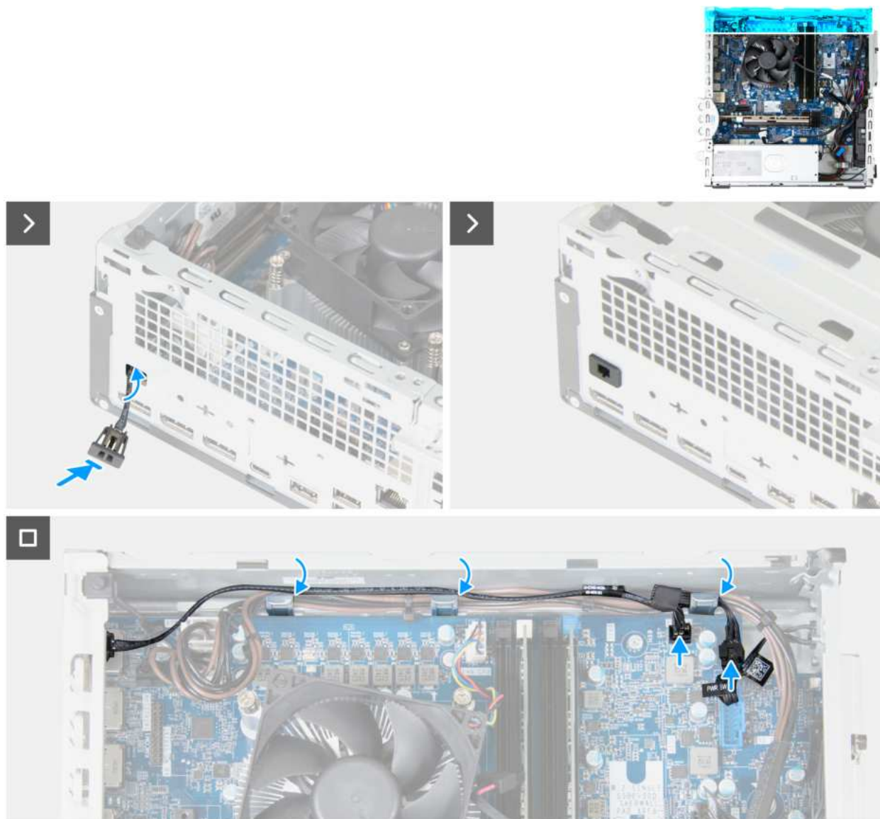
Figure 60. Installing the remote power-switch cable
