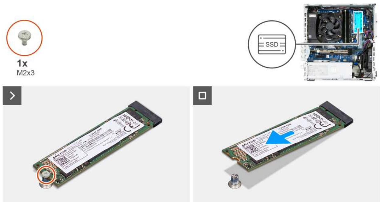
Figure 31. Removing the M.2 2280 solid state drive from slot 2
