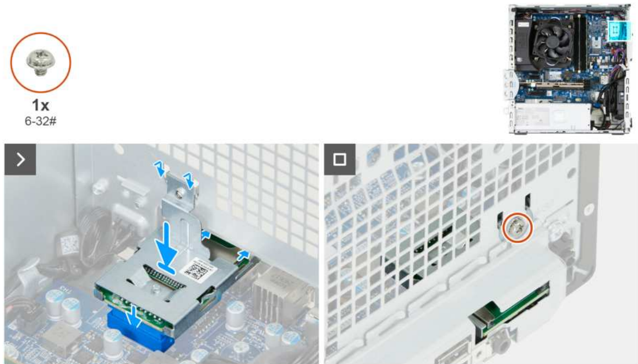
Figure 73. Installing the media-card reader
