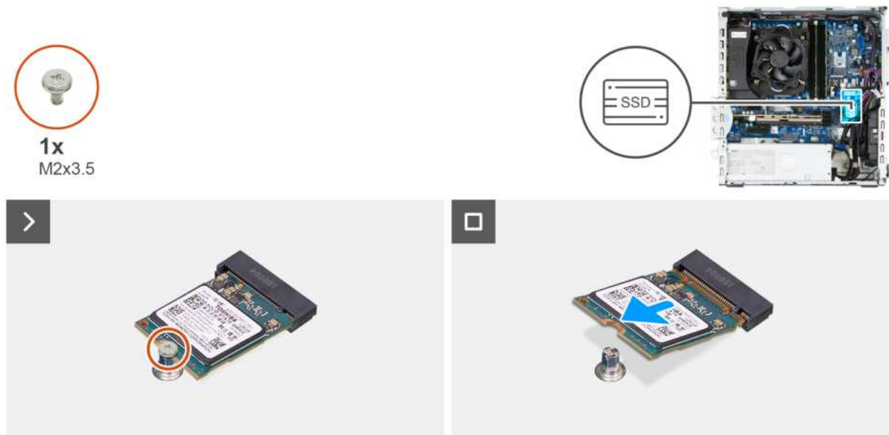
Figure 22. Removing the M.2 2230 solid state drive from slot 0
