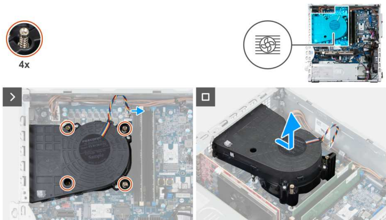
Figure 80. Removing the processor-fan and heat-sink assembly (Dell Pro Slim Plus QBS1250)
