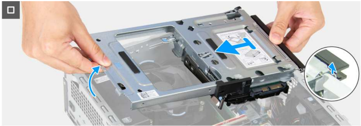
Figure 50. Removing the drive bay
