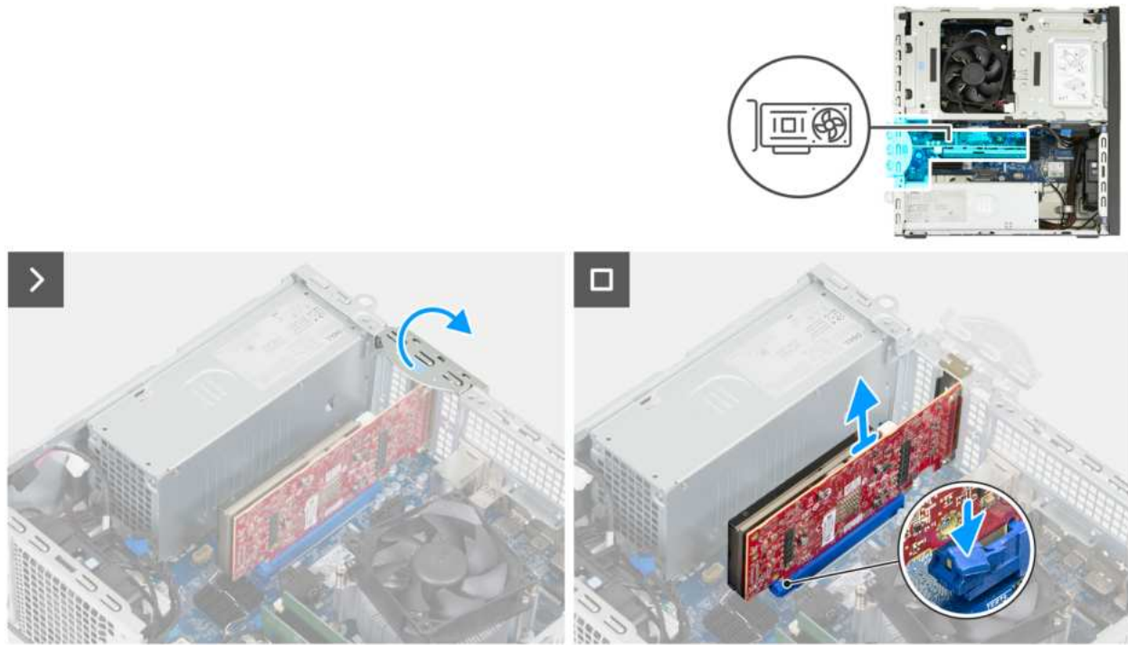
Figure 33. Removing the graphics card
