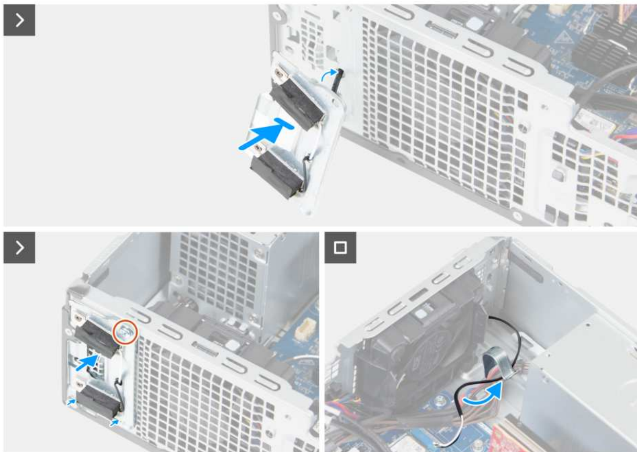
Figure 75. Installing the antenna modules
