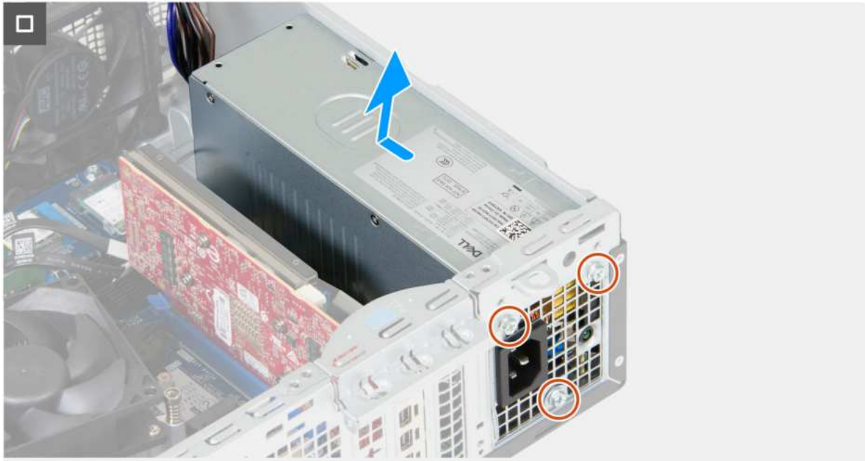
Figure 77. Installing the power-supply unit
