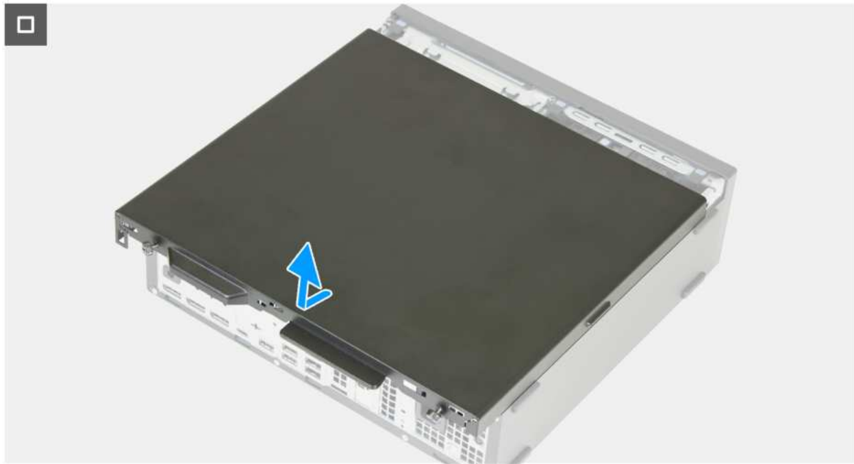
Figure 7. Removing the side cover
