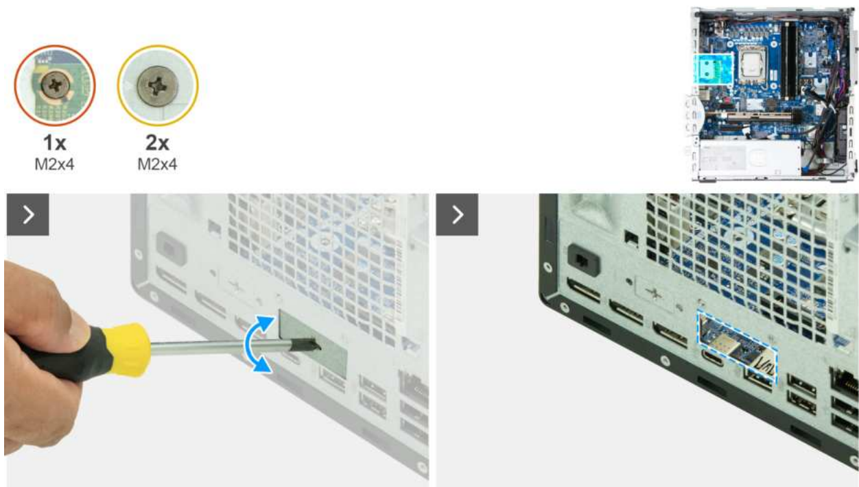
Figure 68. Installing the fiber-optic port module
