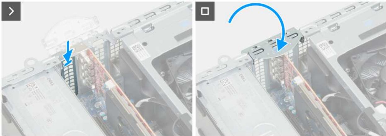
Figure 38. Removing the solid state drive expansion card
