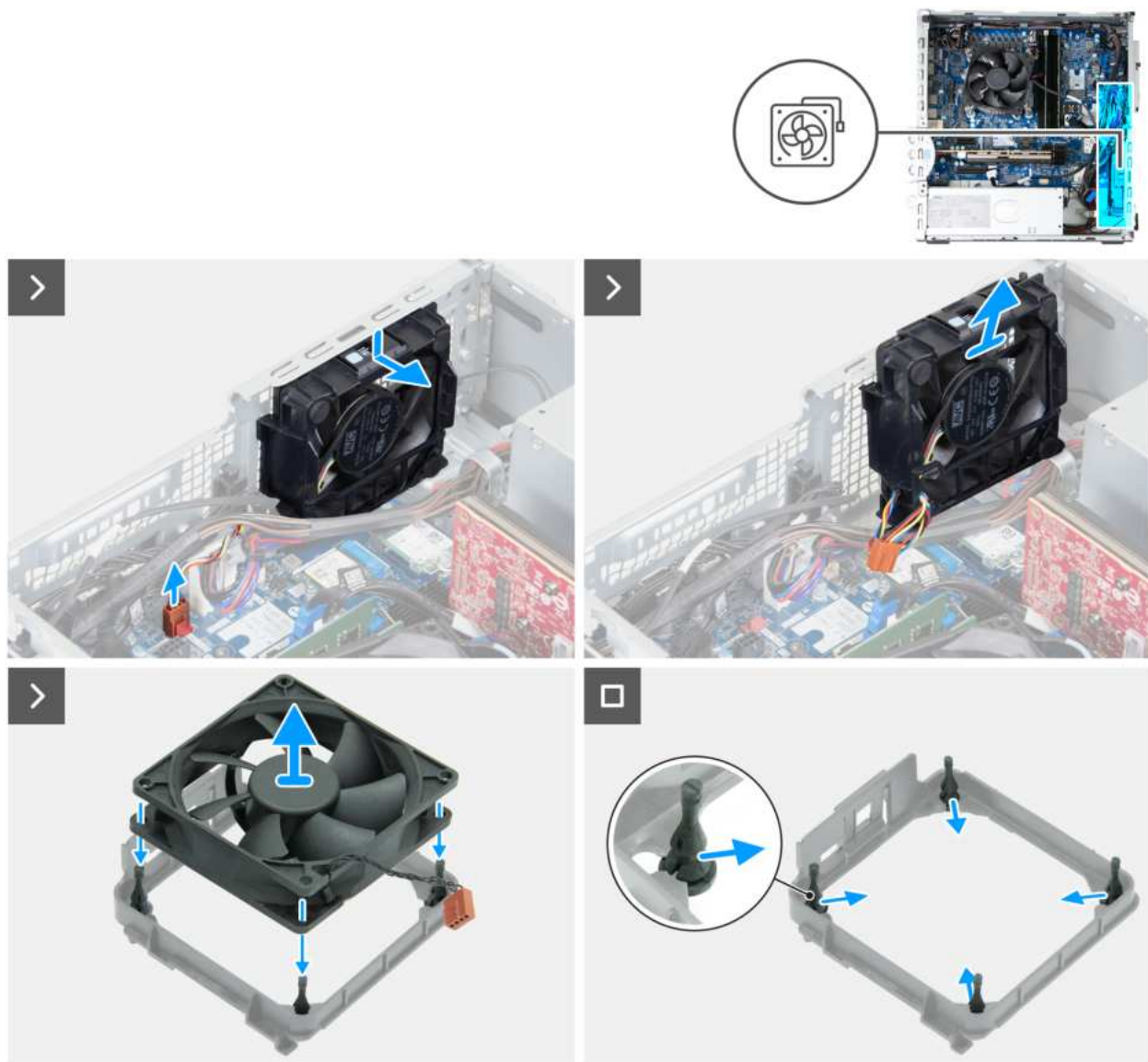
Figure 57. Removing the fan
