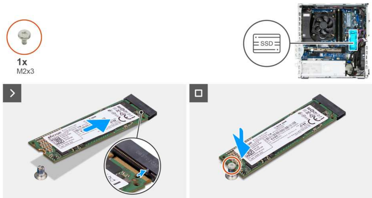
Figure 25. Installing the M.2 2280 solid state drive in slot 0
