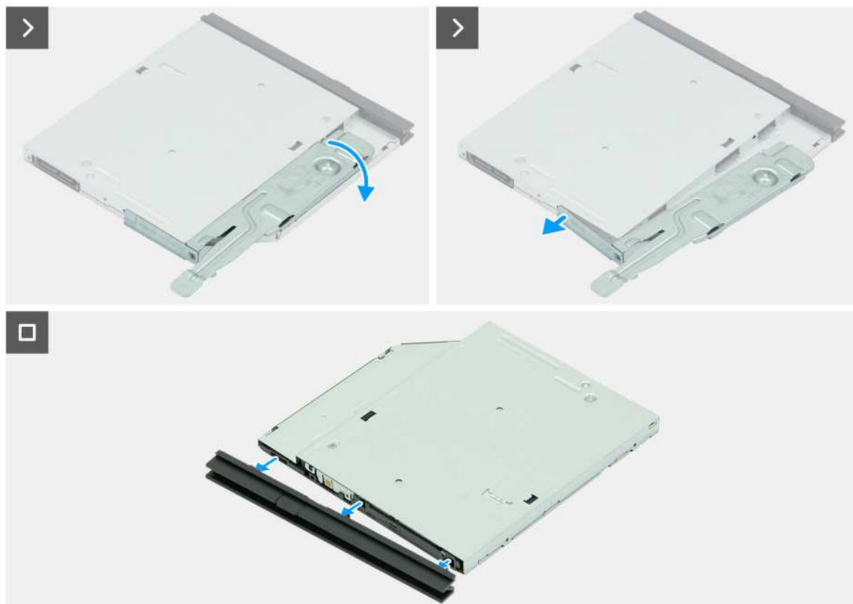
Figure 46. Removing the optical drive
