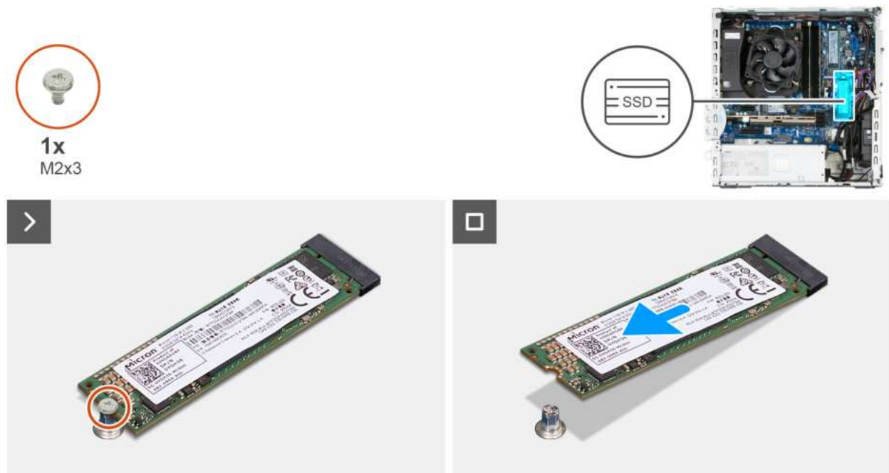
Figure 24. Removing the M.2 2280 solid state drive from slot 0
