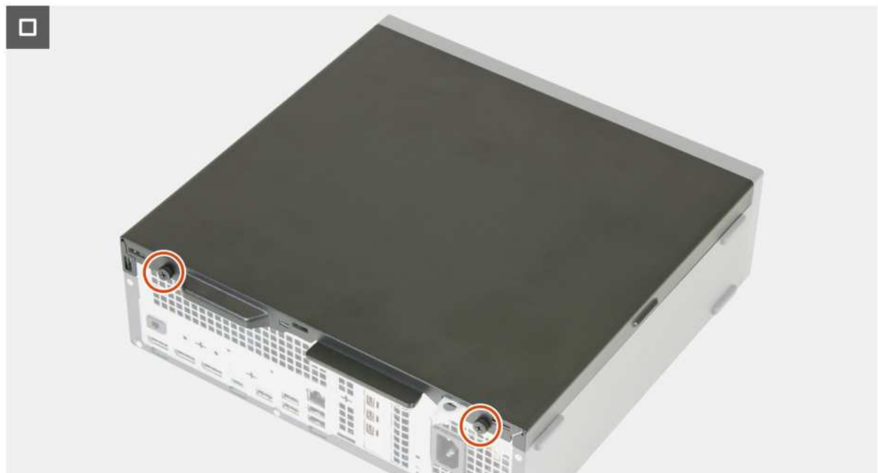
Figure 9. Installing the side cover
