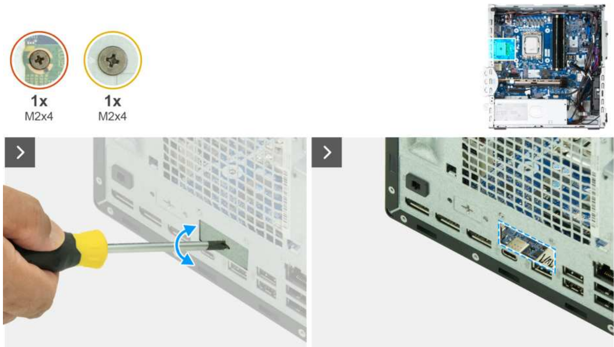
Figure 65. Installing the optional-port module
