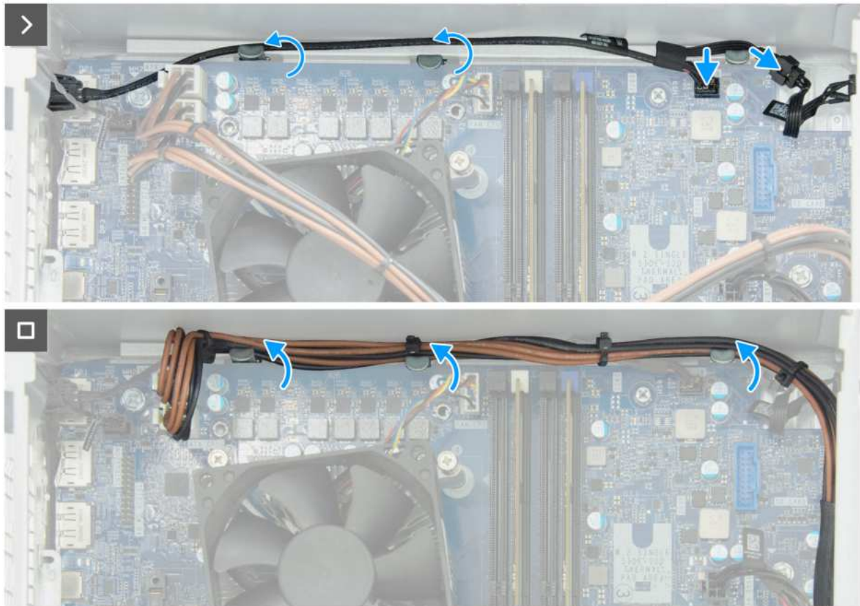
Figure 61. Installing the remote power-switch cable
