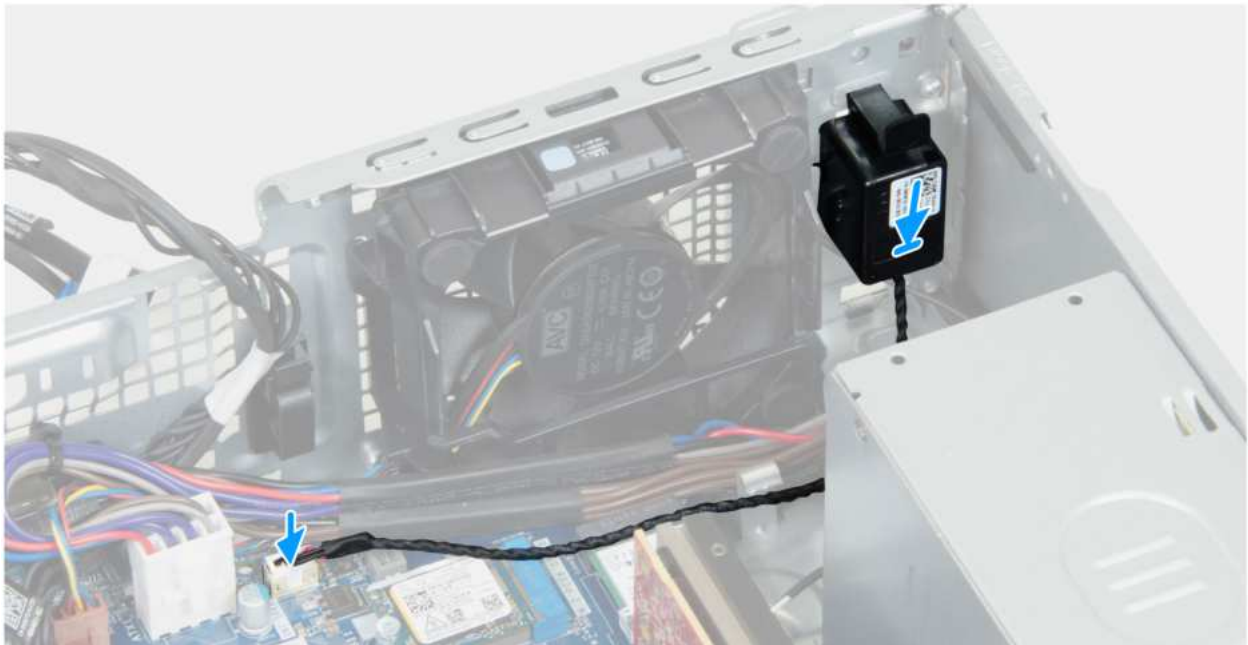
Figure 19. Installing the internal speaker
