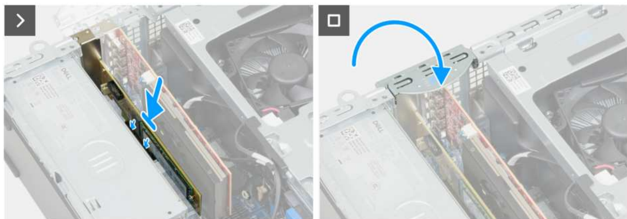
Figure 40. Installing the solid state drive expansion card
