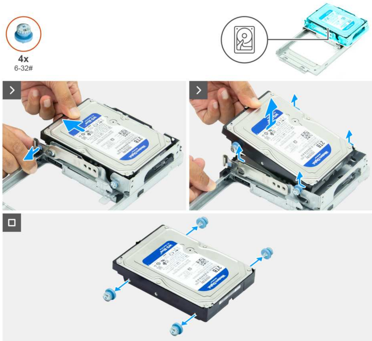
Figure 53. Removing the hard drive
