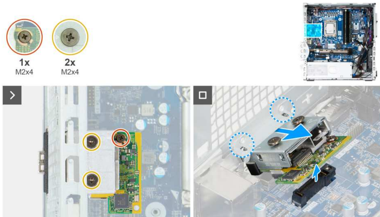
Figure 67. Removing the fiber-optic port module
