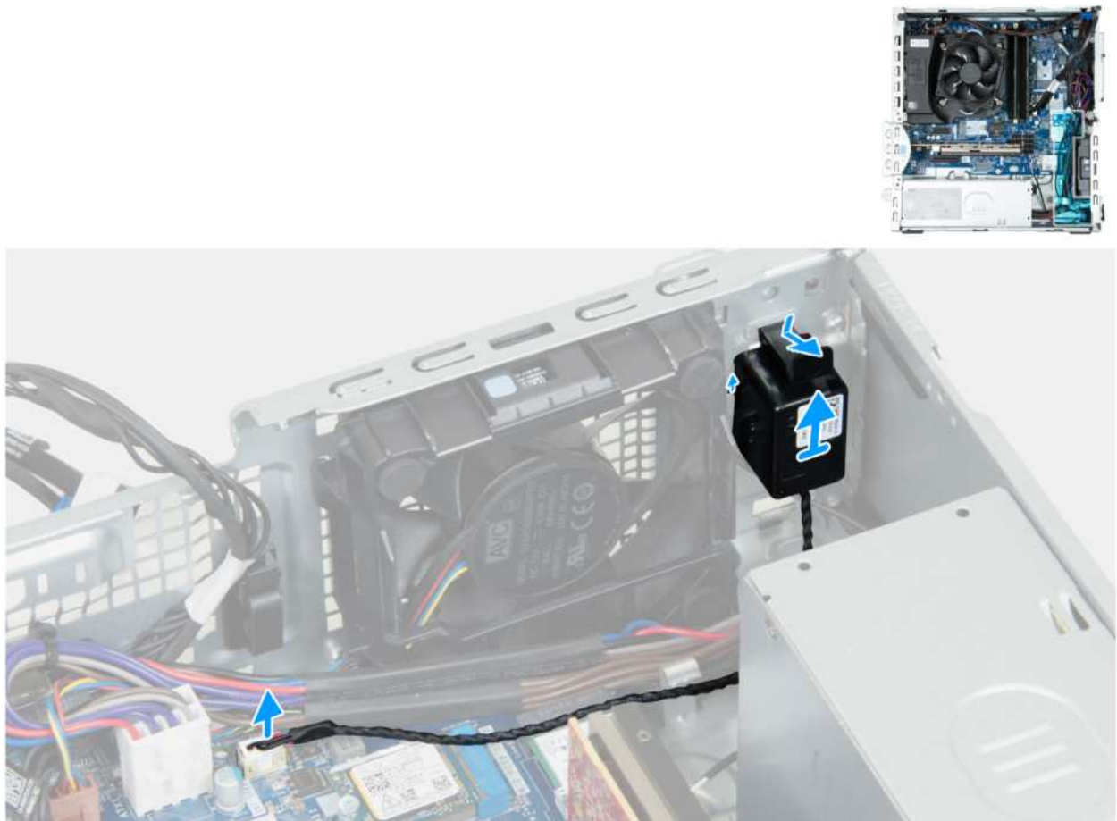
Figure 18. Removing the internal speaker
