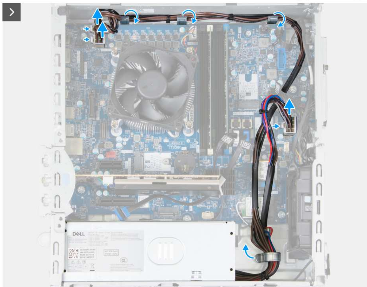
Figure 76. Installing the power-supply unit
