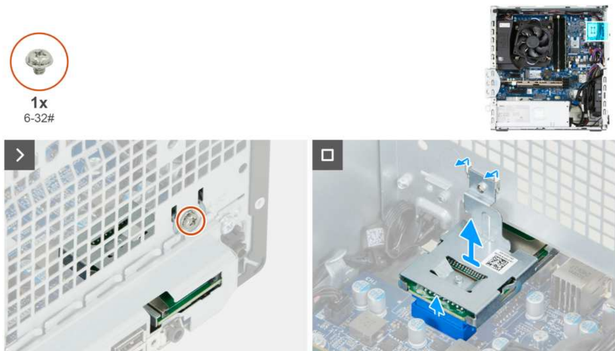
Figure 72. Removing the media-card reader
