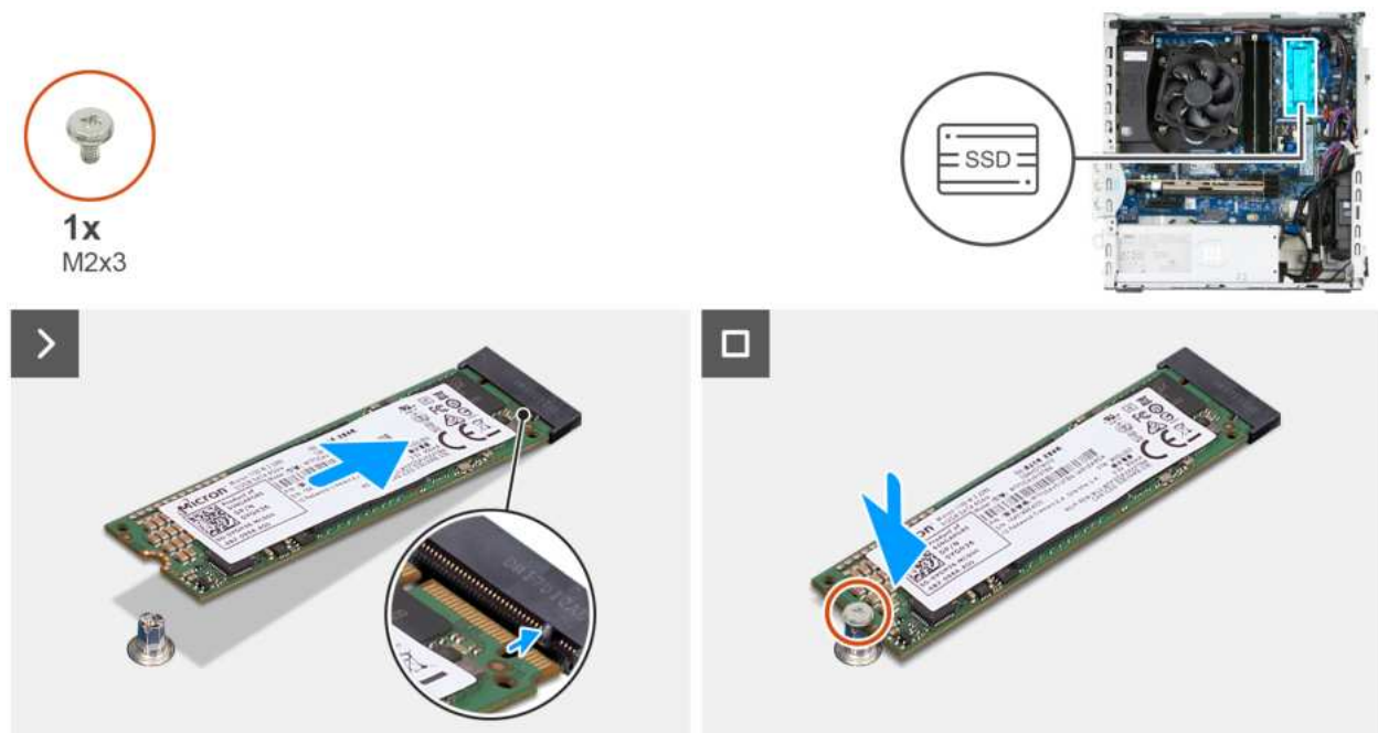
Figure 32. Installing the M.2 2280 solid state drive in slot 2
