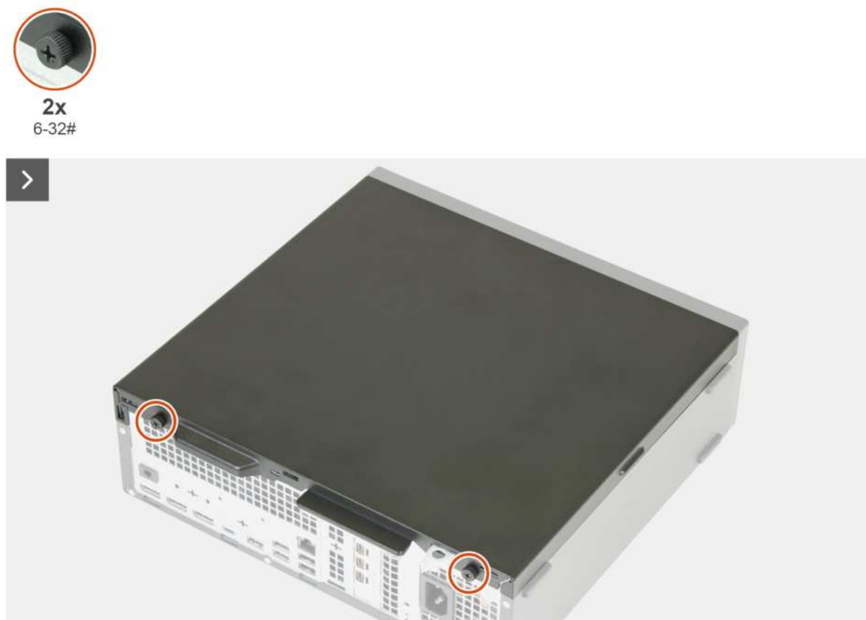
Figure 6. Removing the side cover
