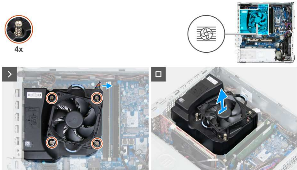
Figure 81. Removing the processor-fan and heat-sink assembly (Dell Pro Slim Plus QBS1250 XE5)
