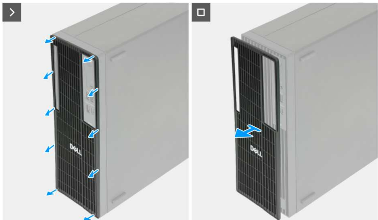
Figure 14. Removing the dust filter
