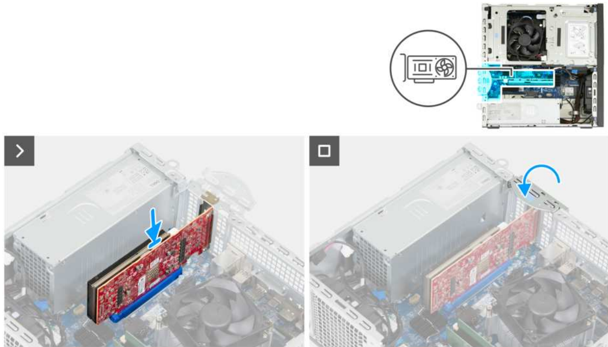
Figure 34. Installing the graphics card
