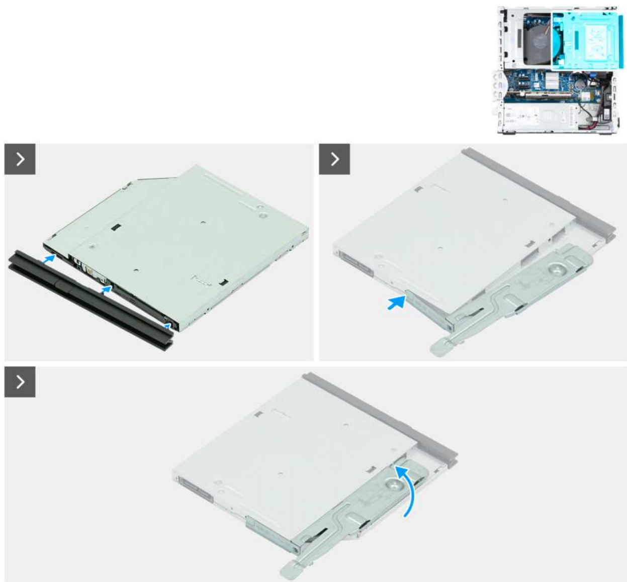
Figure 47. Installing the optical drive
