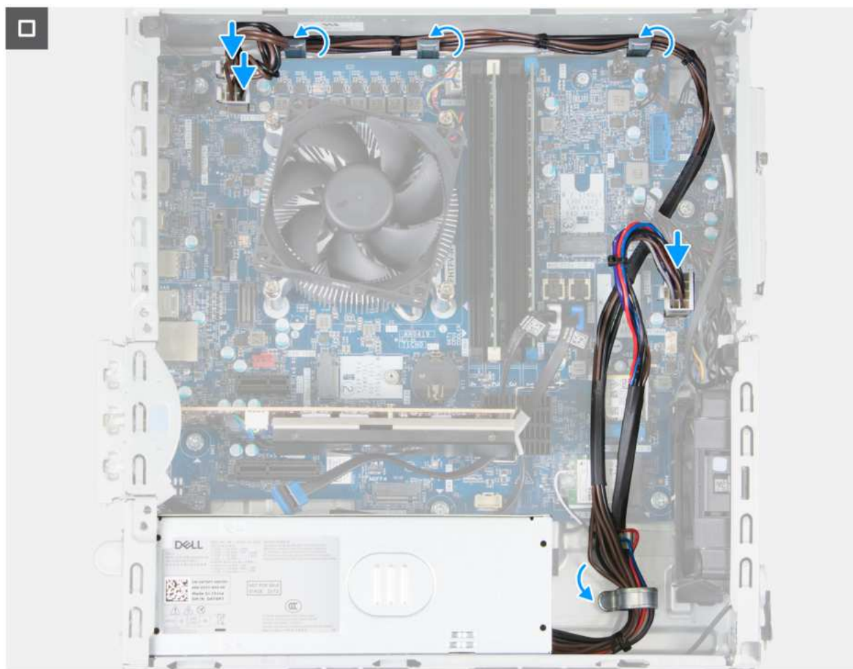
Figure 79. Installing the power-supply unit
