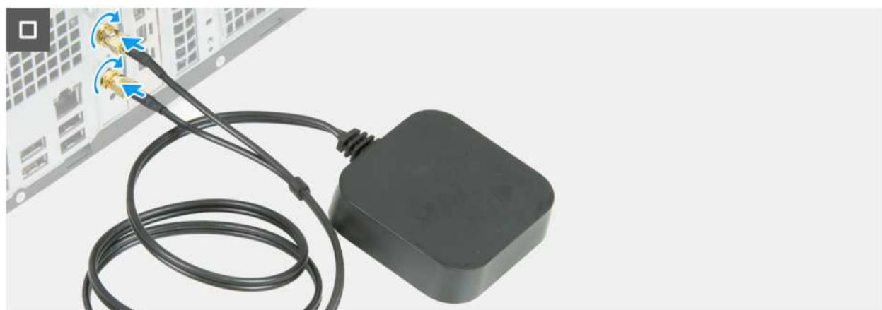
Figure 44. Installing the puck-antenna expansion card
