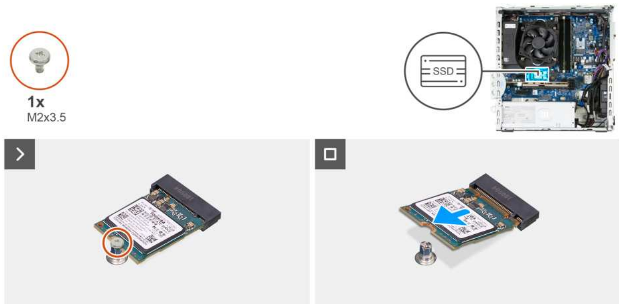
Figure 27. Removing the M.2 2230 solid state drive from slot 1
