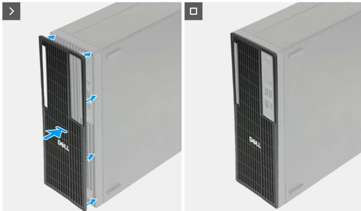
Figure 15. Installing the dust filter
