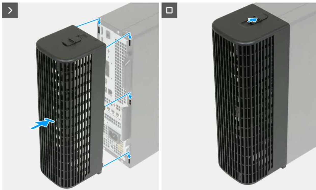
Figure 5. Installing the cable cover
